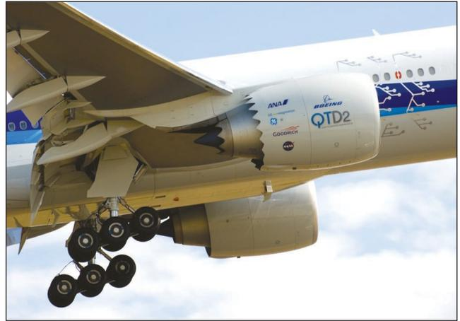
Figure 1. QTD2 engine and landing gear treatment.
