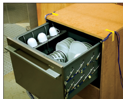
Figure 2. LMS engineers used LMS Test.Lab to perform an acoustic survey using an array of 6 microphones. At the same time, additional microphones localized the background noise levels during operation.
