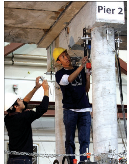
UNR doctoral students Carlos Cruz, left, and Chunli Wei take photos and measurements after the earthquake simulation test.
