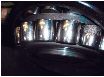
Figure 4. The damaged bearing that caused the potential machinery failure.
