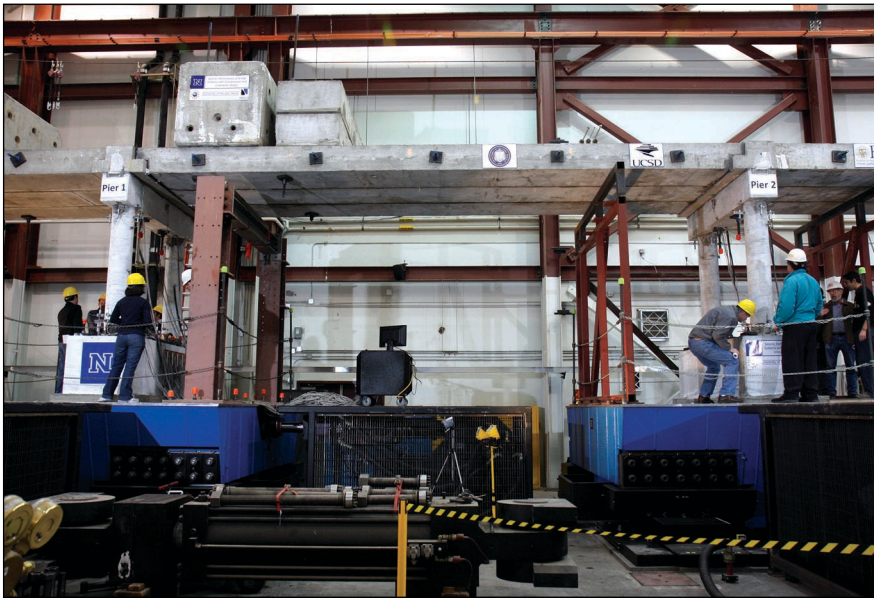
UNR civil engineering researchers and guests look over damage on two of three piers after the earthquake simulation test Dec. 11, 2008. (Photos by Jean Dixon/University Digital Initiatives.)
