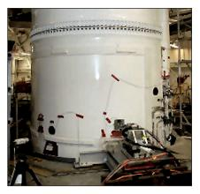
Tap tests were also performed to investigate local modes inside the vehicle. Many of these tap tests utilized m+p international's eight-channel VibPilot system for data acquisition. The modal test data were used to successfully identify and investigate the first four bending mode pairs of the launch vehicle on the mobile launcher platform. These experimental modal parameters were used to calibrate the finite-element model.
