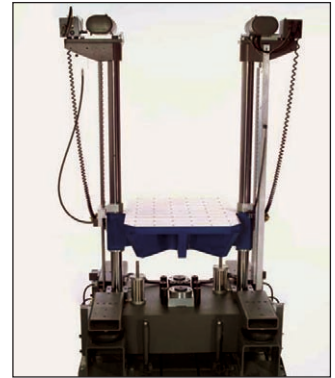
Figure 1. Example of a vertical-drop shock machine.
