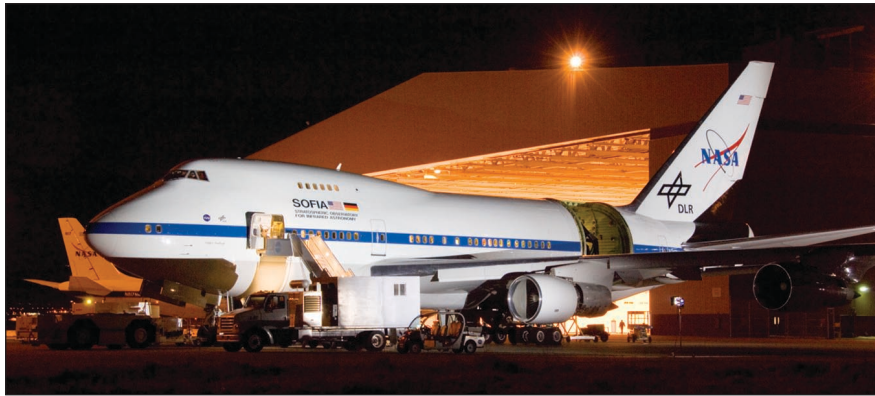
NASA's SOFIA flying observatory during nighttime telescope characterization tests in Palmdale, CA, March 2008.
