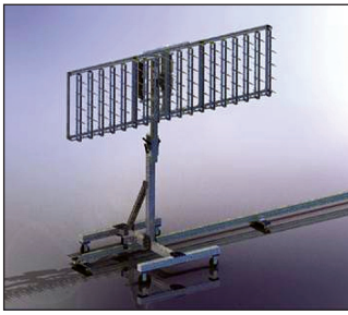
Figure 1. CAD rendering of measurement rig set with the panels in horizontal configuration.
