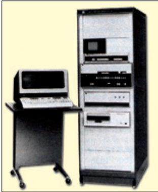
Figure 4. HP5427 vibration control system.
