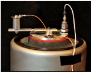
Figure 3. Testing notched beam on a small shaker. Accelerometer (right) mounted on shaker table measures the Control. Cylinder on left is standardized 50-gram mass. Small accelerometer mounted on this mass monitors beam's free-end motion.
