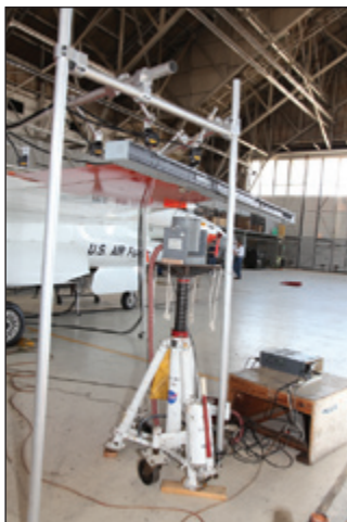
Figure 5. Modal excitation shaker positioned on aircraft structure.
