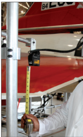
Figure 4. Close-up view of NIRV sensor sighting on aircraft structure.
