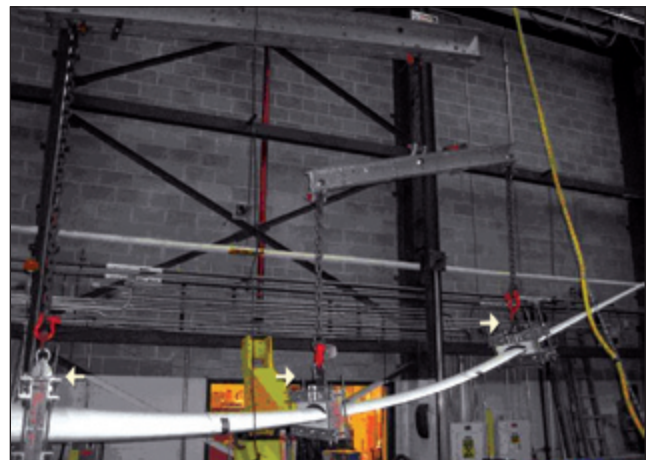
Figure 4. Static test of BSDS wind turbine blade; three-point loading shown at arrows.
