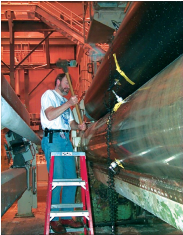
Figure 11. Troubleshooting test to solve self-excitation problem, which was due to thermal baring of rubber roll in paper calendar stack.
