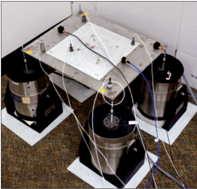
Figure 4. Test plate shown with shakers, stingers and control and measurement accelerometers.
