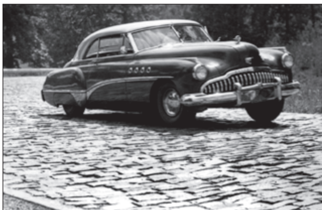
Bangin' a 1949 Buick on the Belgian Blocks – this loop, built in 1929, is one of the most severe suspension tests on the Grounds. The “blocks” can pound under-designed shock-absorbers, bushings and mounts into submission in very short order.
