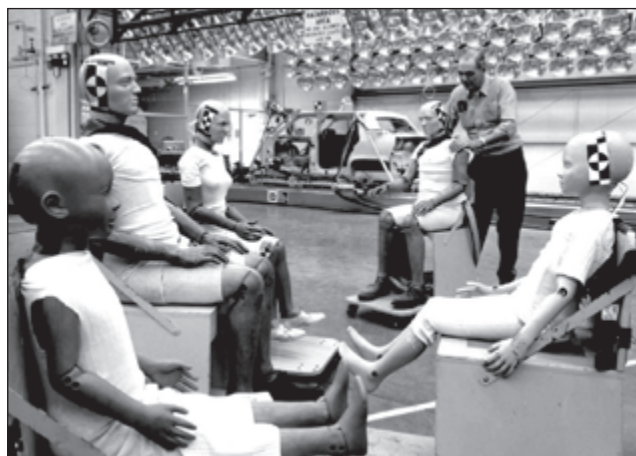
The only dummies who ever worked at the GMPC: the Anthropomorphic Testing Device (ATD) born and bred at GMPC's Safety Research Laboratory for crash testing. A “family” of about 100 ATDs spanning 6-month toddler to 234-lb male adult is always on active duty.
