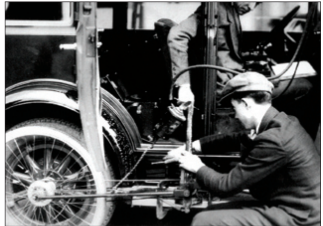
Attaching and adjusting a 1920s era “5th wheel” to accurately measure road speed during a noise test.
