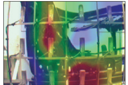
Low-frequency transient noise localization of a car seat frame mounted on a shaker in a normal room.
