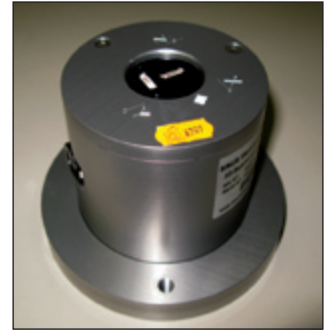
Figure 1. Example of seismometer; weight 3 kg, diameter 120 mm.
