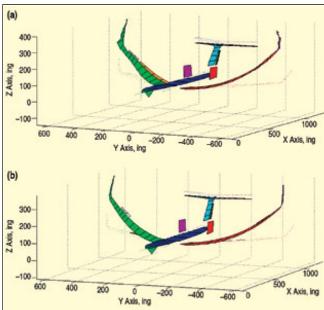
Figure 11. Comparison of test and analysis mode shape results helped test completion decisions.
