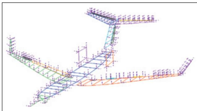
Figure 3. Test display model of the G650; arrows indicate where measurements were made.
