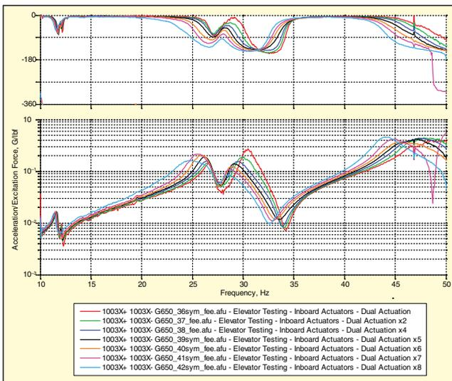
Figure 10. Linearity study of the elevator control surface.
