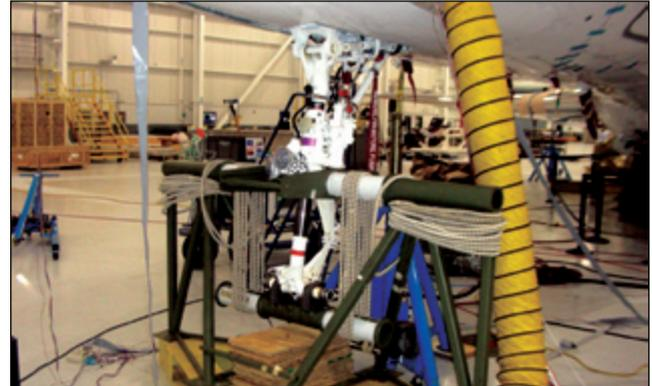
Figure 6. Bungee suspension system installed at nose landing gear.
