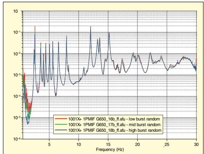
Figure 9. Power mode indicator function used for linearity assessment using multiple excitation levels.
