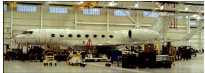
Figure 5. G650 aircraft undergoing GVT.
