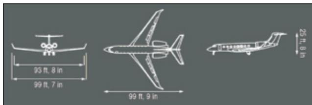
Figure 2. Three-view layout of G650 with dimensions.
