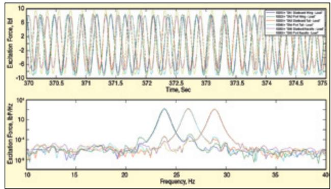
Figure 7. Multi-sine excitation allows for multiple sine sweeps to be conducted simultaneously; excitation forces time domain (top) and spectra (bottom) are shown.
