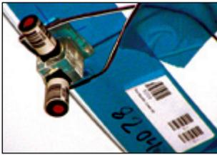
Figure 4. Bar codes placed on sensors and at measurement locations enhance setup.
