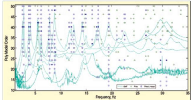
Figure 8. AFPoly stability plot for modal parameter extraction.
