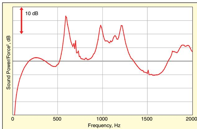
Figure 4. Sound power transfer function for original design.
