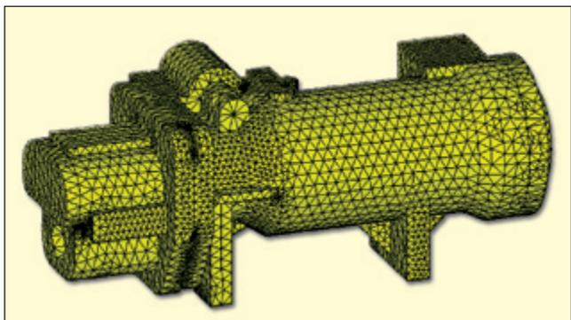
Figure 2. FEM mesh of compressor.
