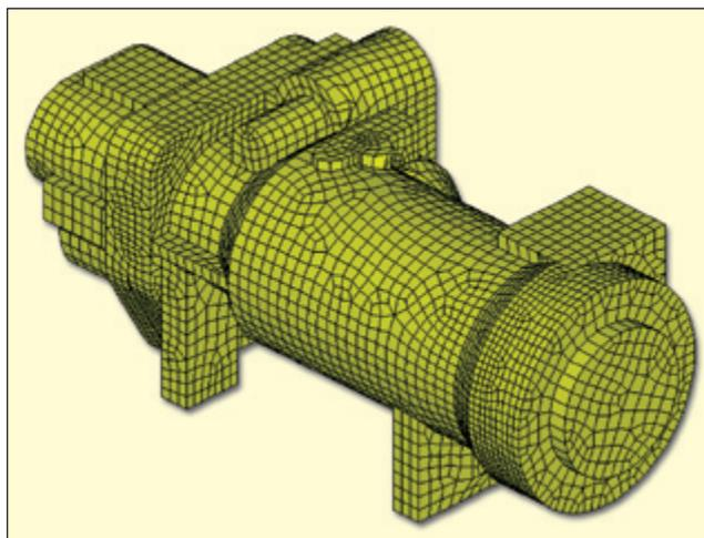
Figure 3. BEM mesh of compressor.
