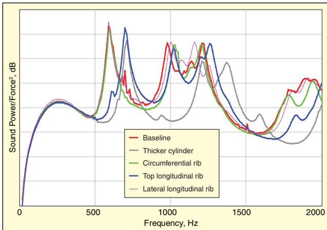
Figure 7. Comparison of sound power transfer functions for baseline and four redesigns.
