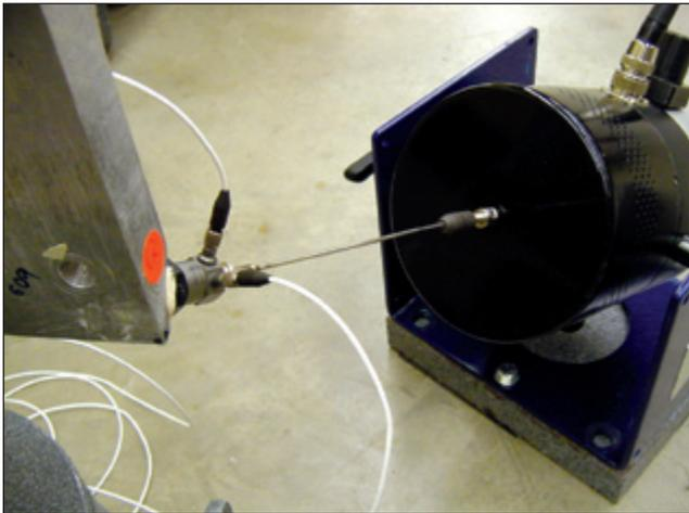
Figure 4. Impedance head mounted in skewed orientation to test structure.
