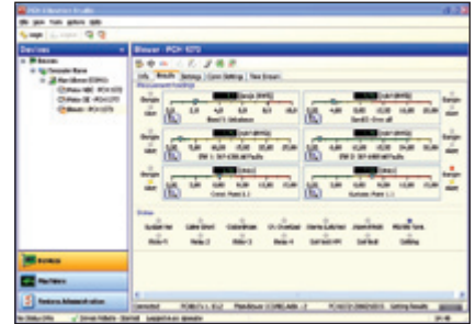
Figure 3. Multi-channel process monitoring system and typical alarm-band display.
