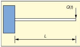
Figure 11. Shallow beam with random tip load.
