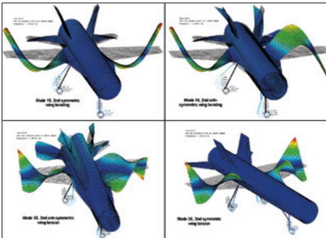
Figure 5. Pseudo-orthogonality of the manual ASET selection indicates that Modes 15, 16, 25, and 26 are not sufficiently represented in the TAM; all four modes are wing modes.
