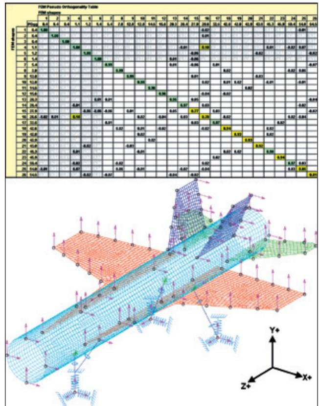
Figure 3. Manually selected ASET; pseudo-orthogonality and FEM are displayed.
