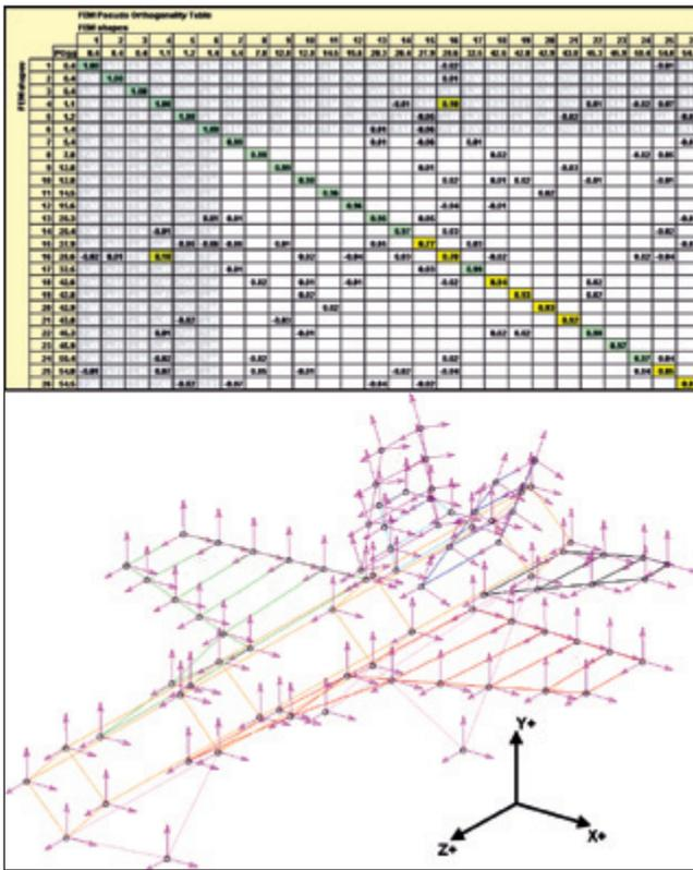
Figure 4. Manually selected ASET, including all three DOFs; pseudo-orthogonality still indicates an insufficient TAM, so a GA reduction would not be productive.
