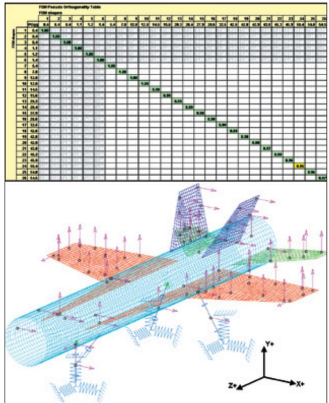
Figure 2. IRKE-selected and GA-reduced 75-DOF ASET; pseudo-orthogonality and FEM are displayed.
