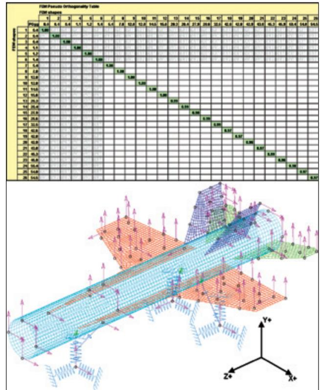
Figure 7. Final ASET, derived from the manual 369-DOF TDM with accelerometers added to the wings and tails and then reduced via GA.
