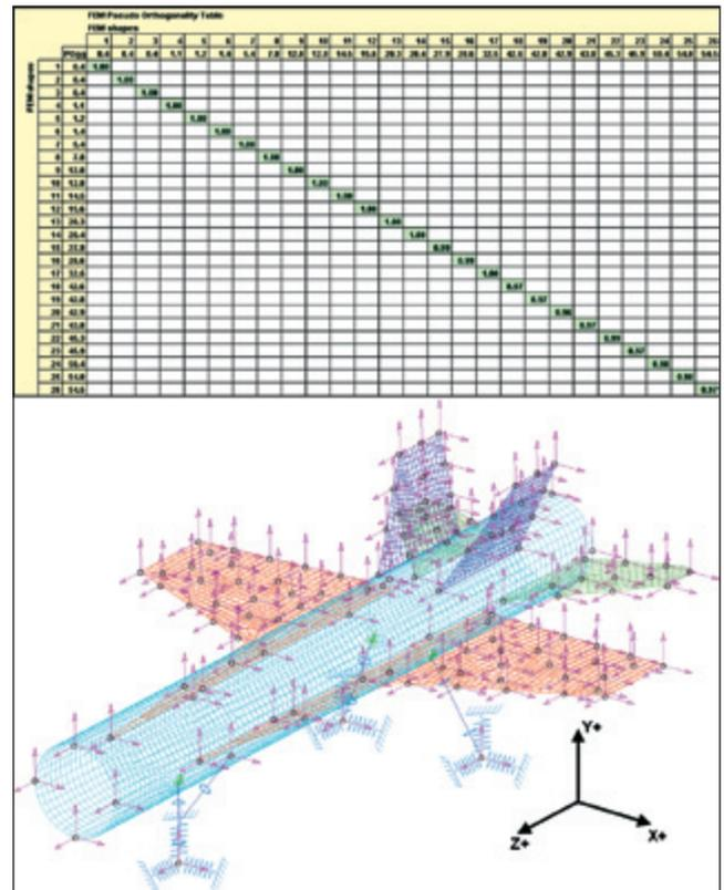
Figure 6. Manually selected ASET, including all three DOFs; additional DOFs were added to the wings and tails, and the pseudo-orthogonality indicates sufficient TAM.
