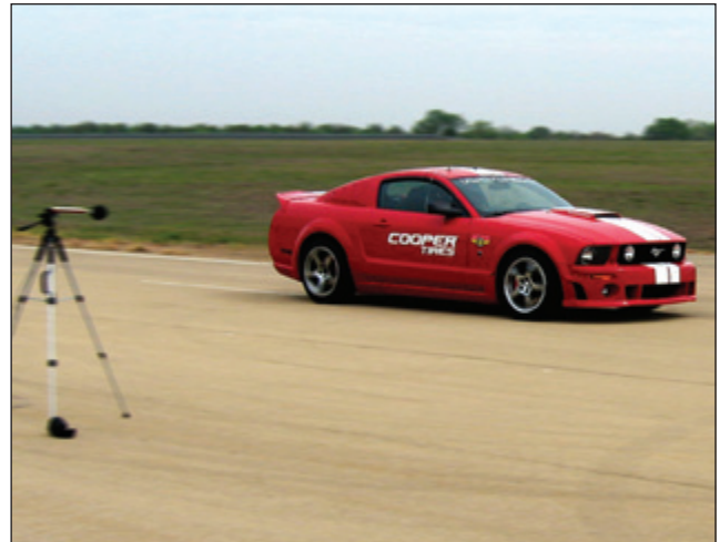
Figure 1. Vehicle triggering measurement with new pass-by noise system.
