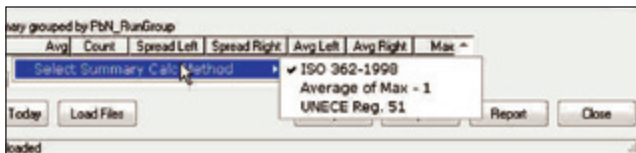
Figure 11. Run summary view allowing operator to compute results using choice of standards.
