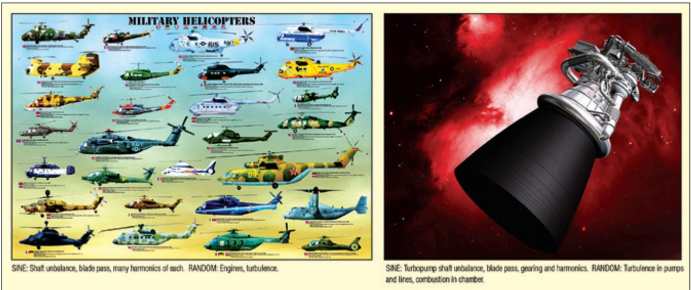
Figure 1. Typical environments that have mixed sine and random elements include helicopters and rocket motors.
