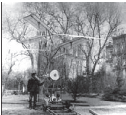
Sikorsky's second helicopter, the S2, was powered by a 25-hp, Anzani motorcycle engine. It lifted briefly (without a pilot) in 1910; the preceding 15-hp S1 could not lift itself.
