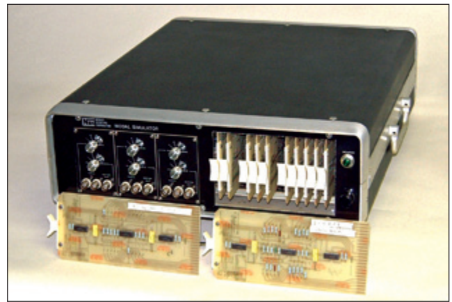
Figure 4. Analog modal simulator built for internal research at Nicolet Scientific Corp. in the late 1970s. Each mode was programmed by soldering selected precision resistors in place. Programming “rules” were printed on the component side of a two-layer PC. Card on left holds a real-mode shape; one on right defines complex mode. Each card contained coefficients for 5 degrees of freedom. Simulated frequency response function could contain as many modes as there were cards plugged into frame. BNCs and rotary switches at left allowed simultaneous excitation up to three DOFs and simultaneous displacement measurement at same or three other DOFs. Results were analyzed using the Nicolet 660 series FFT analyzer, a highly capable two-channel instrument.
