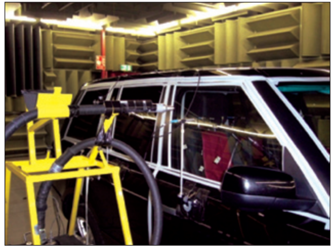
Figure 4. High-frequency acoustic volume velocity source applied outside vehicle front side glass.
