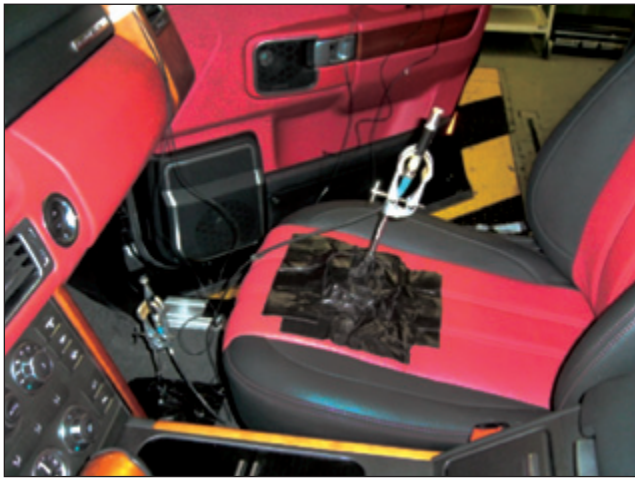
Figure 2. Microphones at lower positions to measure cabin SPL distribution and acoustic transfer functions involving lower interior positions.
