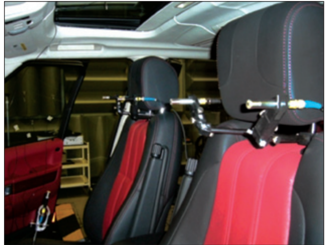
Figure 1. Standard inner- and outer-ear microphone positions to measure SPL for driver and front passenger locations.
