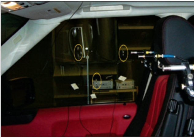
Figure 6. Three accelerometers mounted on vehicle front side glass.
