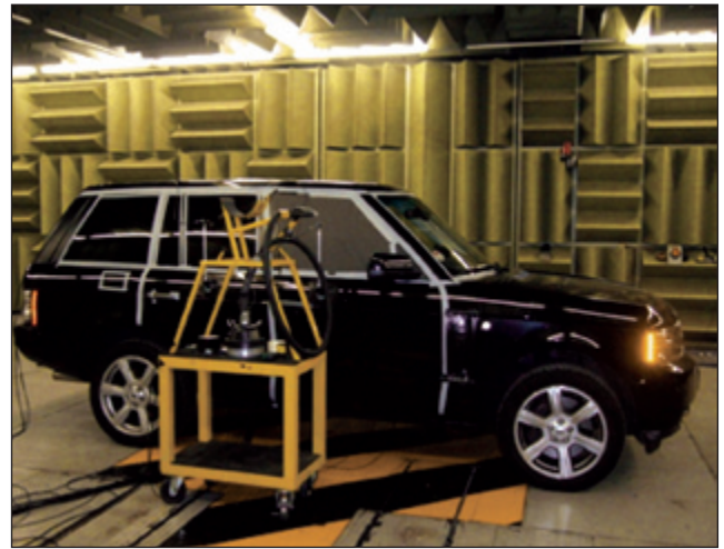
Figure 14. Use of heavy layer to confirm effect of blocking dominant transmission path.
