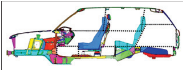
Figure 3. Side-view illustration of typical subdivision of interior cabin airspaces in SEA Model.
