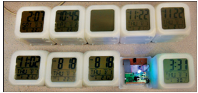
Figure 6. Ten of the clocks after testing; one completely failed LCD.
