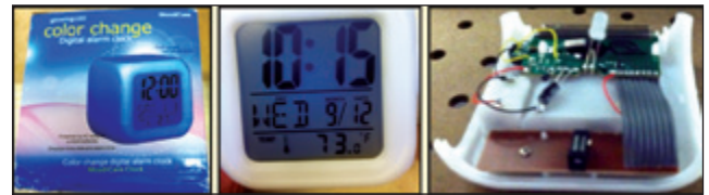
Figure 1. Details of the 12 digital clocks used as the devices under test.
