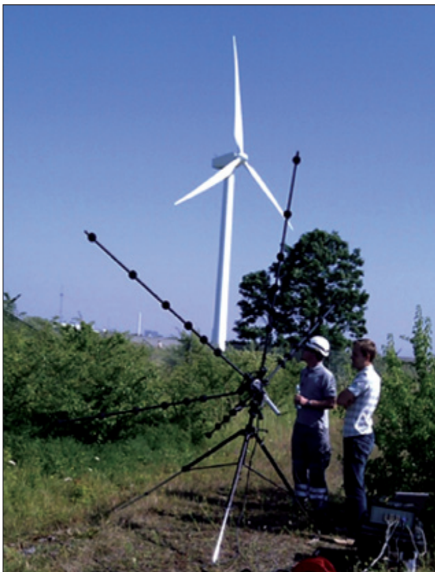
Figure 10. Pentangle array for field measurement of large structures and for moving noise sources.
