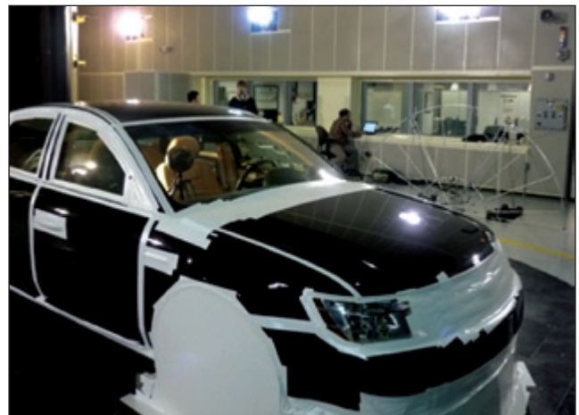
Figure 6. Wind tunnel with taped vehicle on rotating plate used to adjust yaw angle; spherical beamformer in the cabin and half-wheel beamforming array at 3.8 m distance (0 degree yaw).
