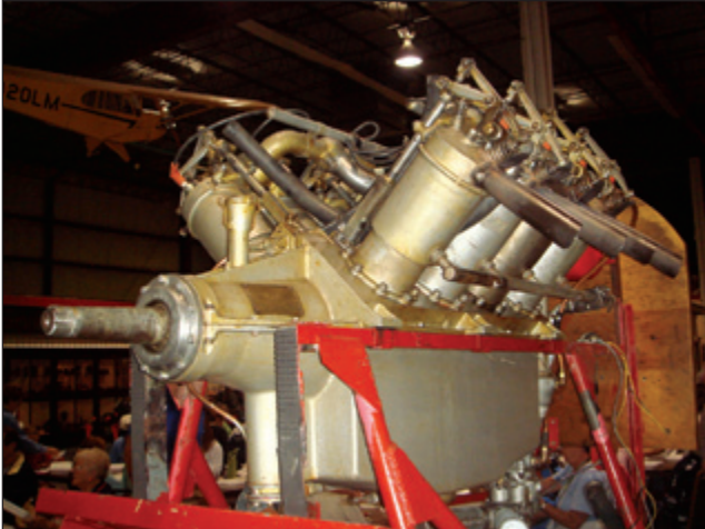
Figure 9. An original OX-5, 90 HP, water-cooled V-8 engine used to power a reproduction of the A-1 Triad (land-sea-air) flying boat.
