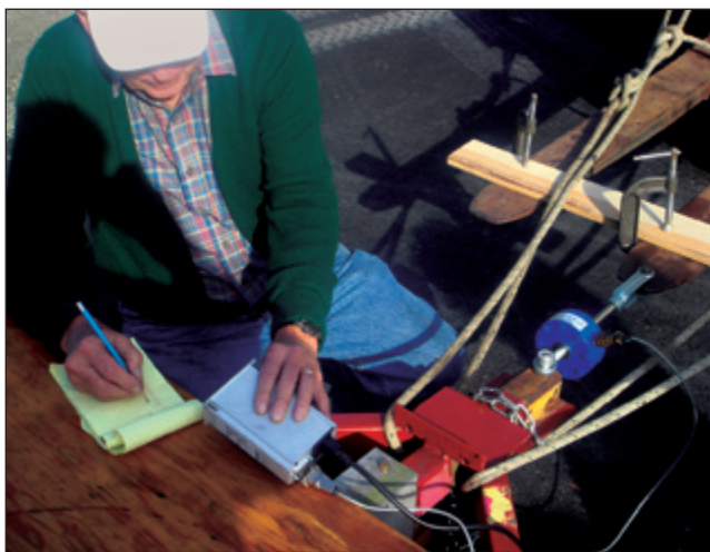
Figure 5. Brian Grigsby takes thrust measurements using a PCB load cell and digital readout meter.
