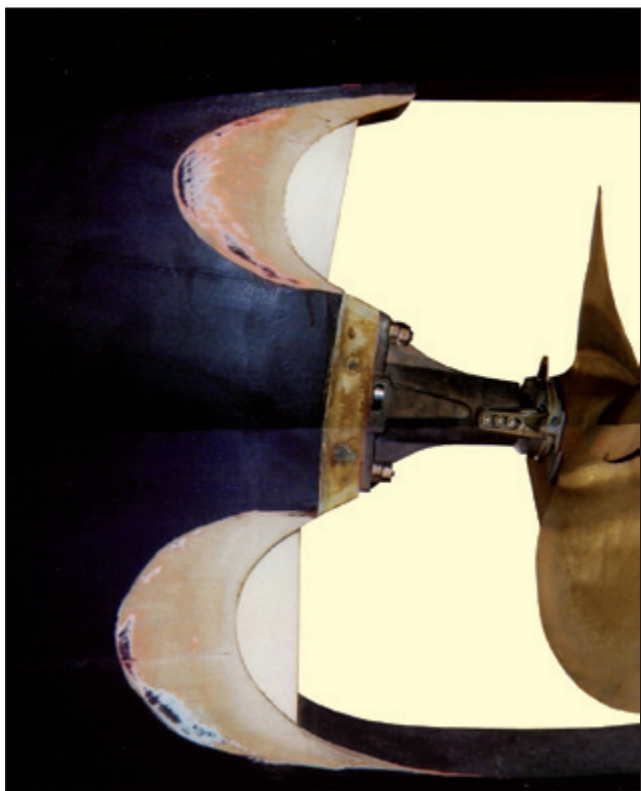
Figure 3. Propeller shaft and keel of fishing boat. Note the “half-moon shaped” blocks above and below the cutlass bearing. After these blocks had been installed, the hull and deck vibration went down dramatically.
