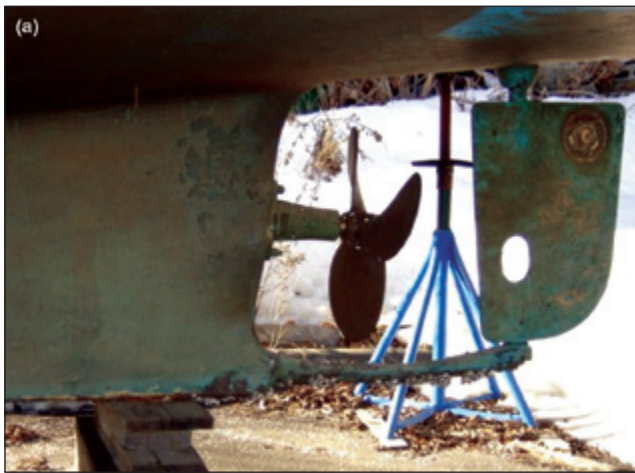
Figure 1. Propeller shafts on single- and twin-engine vessels. Note that on the single engine (a), the propeller shaft comes out of the keel and is relatively well protected by the keel. On the twin engine vessel (b), the shafts come out from the hull and are supported by struts. In this configuration, the propellers and shafts are not well protected.
