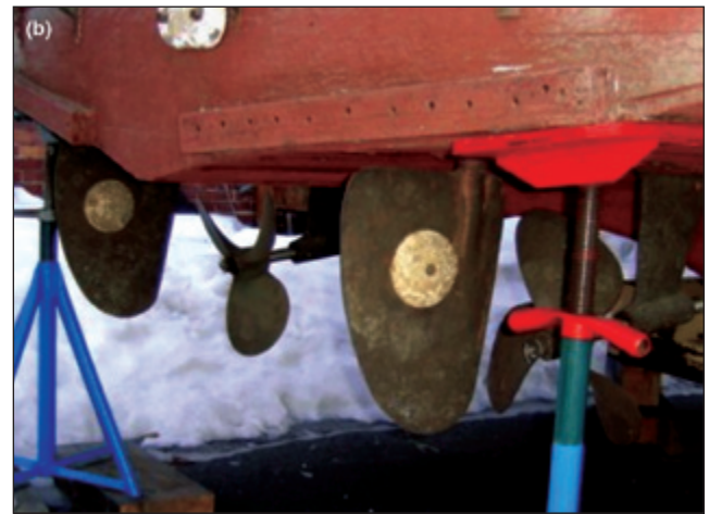
Figure 1. Propeller shafts on single- and twin-engine vessels. Note that on the single engine (a), the propeller shaft comes out of the keel and is relatively well protected by the keel. On the twin engine vessel (b), the shafts come out from the hull and are supported by struts. In this configuration, the propellers and shafts are not well protected.
