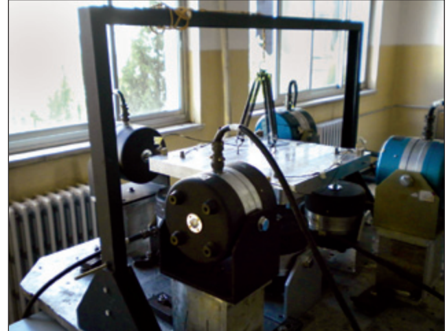
Figure 7. Customer-assembled six-DOF system using 2-2-4 configuration.
