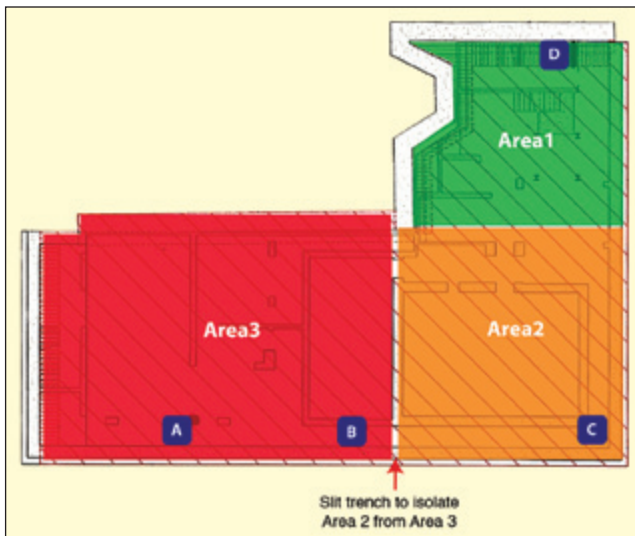
Figure 5. Location of measurement points on slab.
