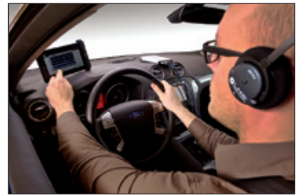
LMS SCADAS XS being monitored using an LMS Smart Scope on the dash panel and LMS 3D Binaural Headset.
