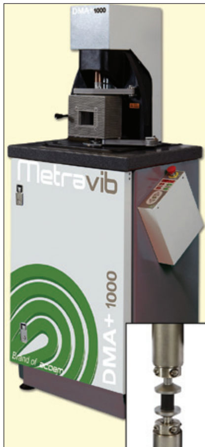
Figure 2. Metravib Dynamic Analysis System and close-up of sample fixture.
