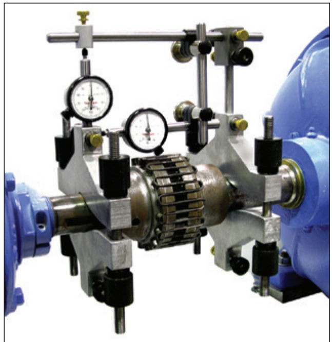
Figure 8. Typical shaft alignment test setup.
