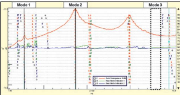
Figure 12. Stability diagram from OMA test with restricted impacts at the node of the third flap-wise mode of the structure.
