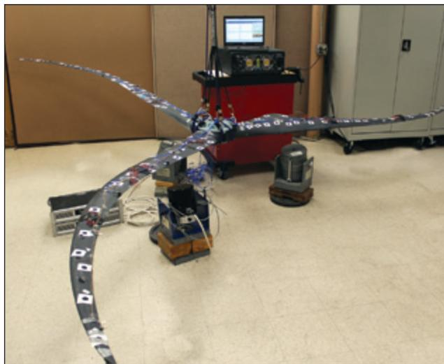
Figure 1. Three-bladed wind turbine system in free-free configuration tested using EMA, OMA, and hybrid techniques.
