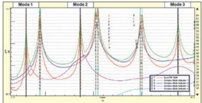
Figure 9. Stability diagram from MIMO test showing first three collective flap-wise modes of wind turbine structure.
