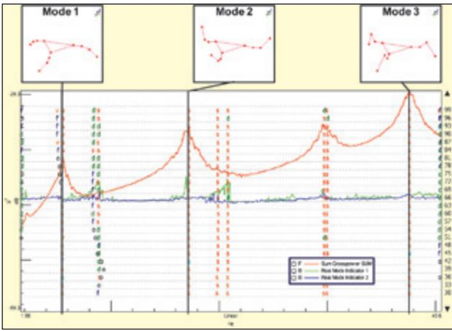
Figure 11. Mode shapes and stability diagram for OMA test on three-bladed wind turbine.
