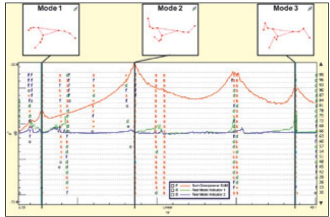
Figure 13. Characteristic mode shapes and stability diagram of three-bladed wind turbine found through hybrid EMA and OMA test using four-shaker random input excitation and restricted-impact excitation at nodes of third flap-wise mode.
