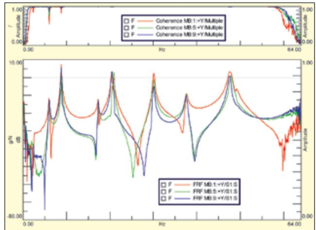
Figure 8. Typical FRF measurements of three-bladed wind turbine structure from traditional shaker modal tests (MIMO).
