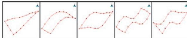
Figure 4. Typical first five mode shapes from four-shaker MIMO tests of frame.
