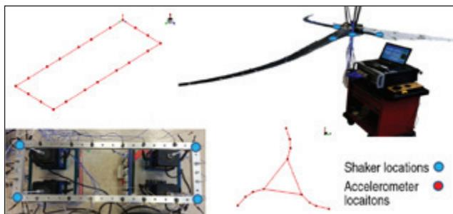
Figure 2. Experimental setup of tested structures showing locations of accelerometers and shakers.
