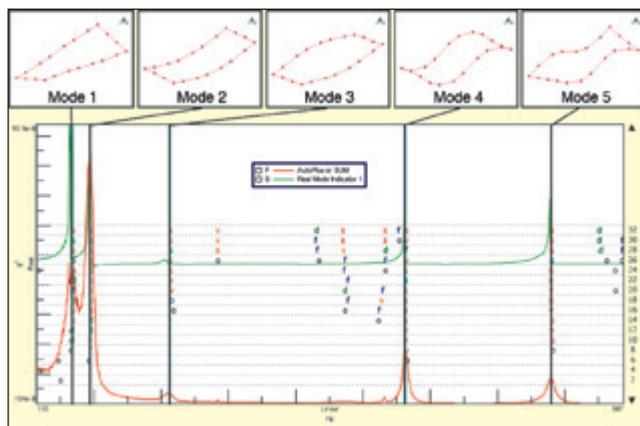
Figure 5. Mode shapes and stability diagram for OMA test on frame.
