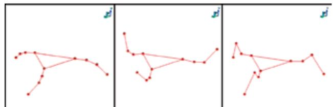
Figure 10. Typical first three flap-wise mode shapes from four-shaker MIMO tests of wind turbine structure.
