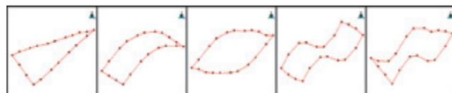
Figure 7. Characteristic operating shapes of frame found through hybrid EMA and OMA test using four-shaker random input excitation and restricted impact excitation at nodes of first torsion mode.
