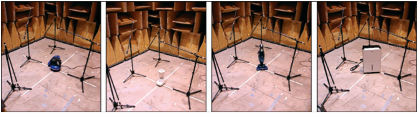
Figure 3. Common household sound sources from left-to-right: 100-psi air compressor, blender/mixer, cordless boom/vacuum, and dehumidifier; sources shown in the ARL/Penn State hemi-anechoic chamber with four PCB 378B02 microphones.
