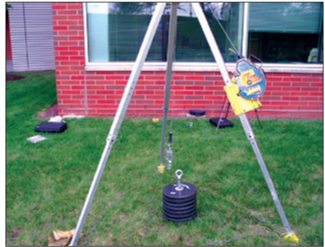
Figure 3. 200-pound drop-weight apparatus.
