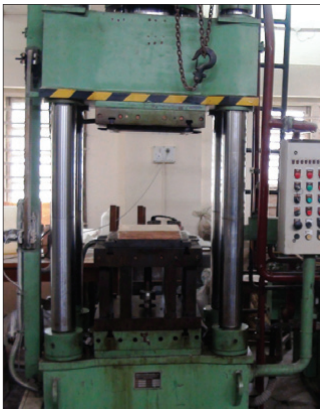
Figure 2a. 300-ton hydraulic press used for compression moulding.
