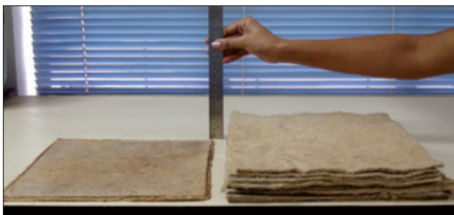
Figure 2b. Chemically treated jute felt before and after the compression.
