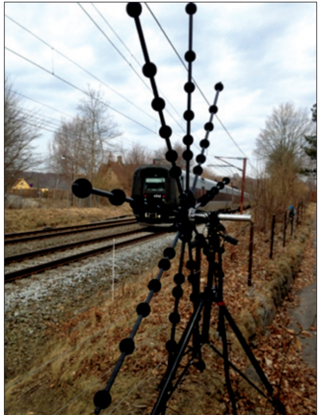
Figure 15. Logarithmic wheel array with 56 microphones and nine arms used for measurements on trains.
