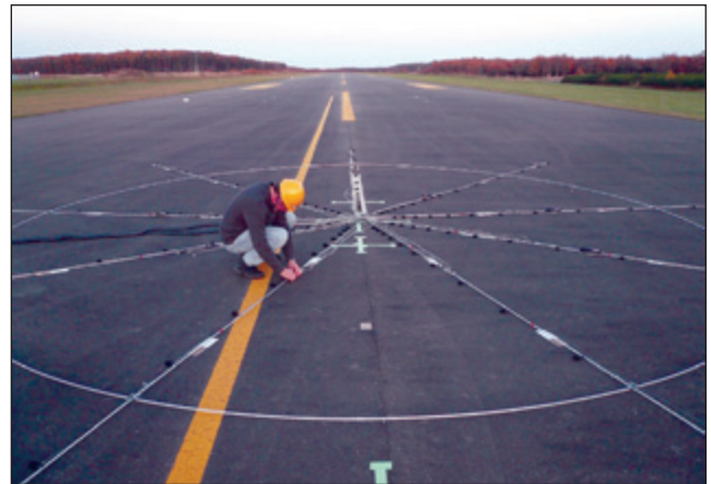
Figure 22. Array on runway is 12 meters in diameter with nine radial arrays, each with 12 microphones (108 total).
