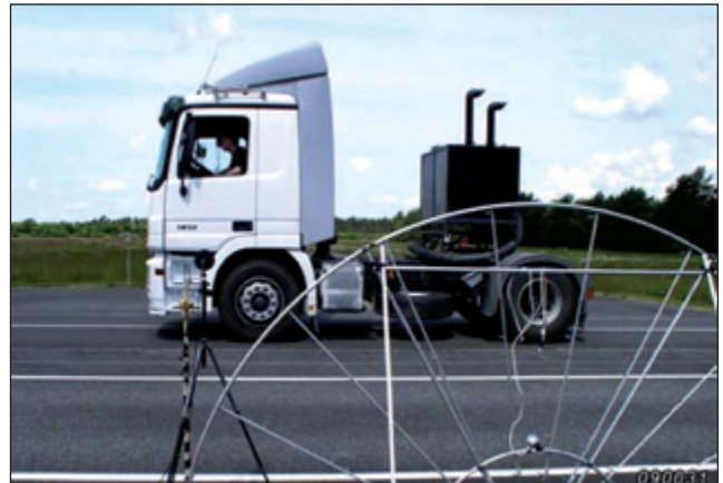
Figure 8. Truck and half wheel array on test track for road vehicle moving-source beamforming measurements.
