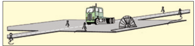
Figure 6. Typical setup for road vehicle moving-source beamforming – array, photocells and radar.
