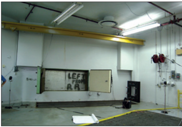
Figure 3. Reverberation room side of original STL opening showing the backside of removable anechoic wedges and the original STL fixture (on floor, to far right).
