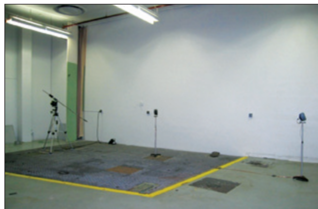
Figure 1. Original reverberation room with open floor grating covering below-floor pit, floor-to-ceiling corner drapery enclosure, and retracted drapery.
