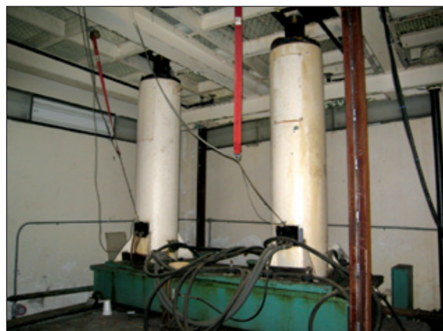
Figure 2. Original pit below reverberation room with four-post vehicle shaker.
