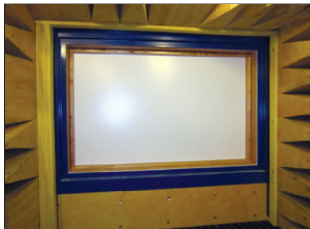
Figure 7. Anechoic room side view of the STL opening showing revised anechoic wedges surrounding opening and physical access behind the opening.
