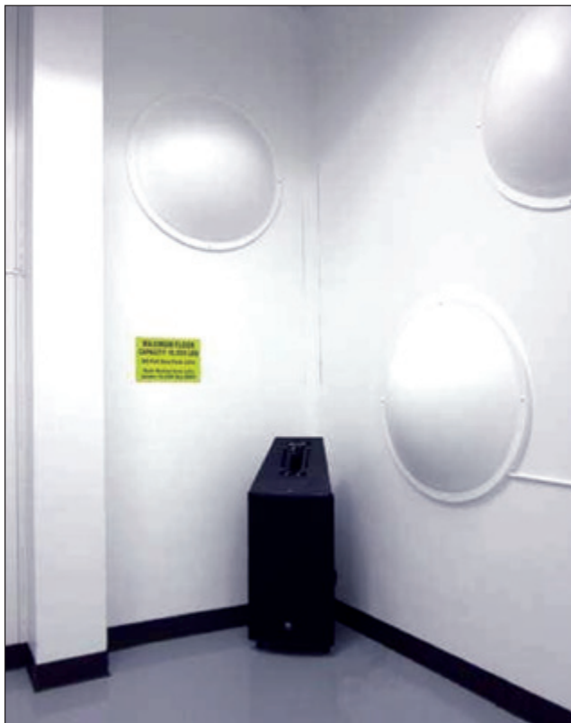
Figure 9. High-power loudspeaker system located in one corner opposite the STL opening (along with three stationary diffusers).
