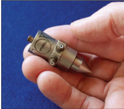
The seemingly forgotten impedance head – one of the greatest tools for understanding vibration phenomena.
