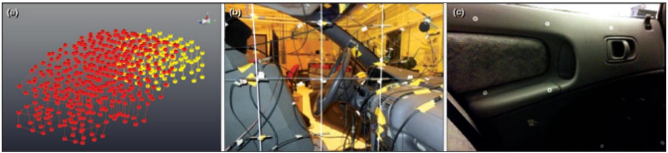
Figure 13. Measurement points. (a) Test model derived from CAE model with markers indicating all microphone locations; (b) Array of microphones inside the cavity; (c) Measurement locations on boundary surface.
