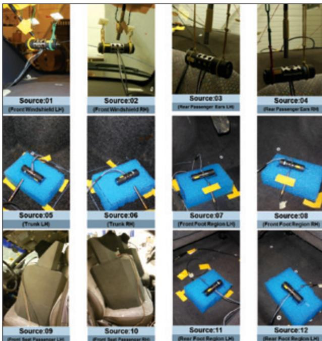
Figure 15. Detailed view of source locations and used sources.
