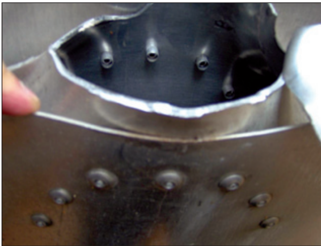
Figure 5. Close up of stress fracture separation from fan hub.
