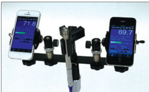
Figure 1. The SoundMeter app on iPhone 5 (left) and iPhone 4S (right) compared to half-inch Larson-Davis 2559 random incidence Type 1 microphone (center).
