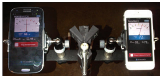
Figure 4. NoiseWatch app on the Samsung S3 Android device (left) and the iPhone 5 (right).
