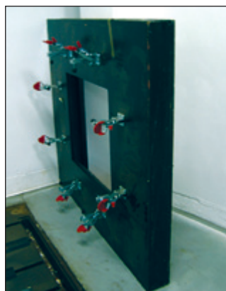
Figure 2. Previous flat sample STL holding fixture.
