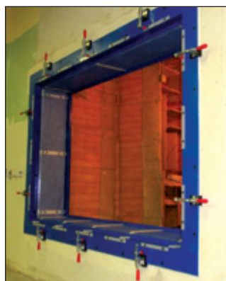
Figure 3. Reverberation room side of the matching plate steel perimeter frames showing perforated protective facing that covers center sound absorption and clamps that secure interchangeable inserts.
