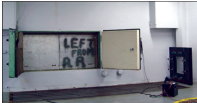
Figure 1. Original STL opening between the reverberation room and anechoic room.
