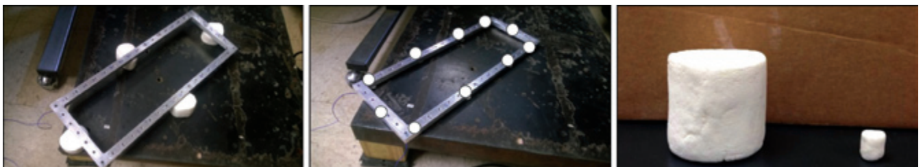
Figure 1. Testing configuration for aluminum frame on four large marshmallows and on 10 small marshmallows.
