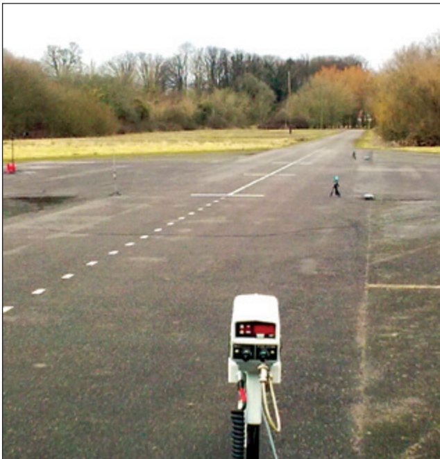
Figure 3. Radar and light gates to determine vehicle position and speed.
