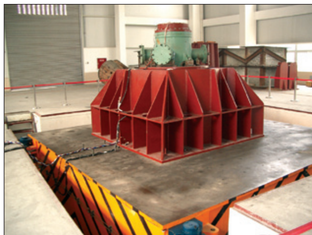
Figure 1. 6 meter x 6 meter seismic table with eight actuators – 4 Z, 2 X, 2 Y.
