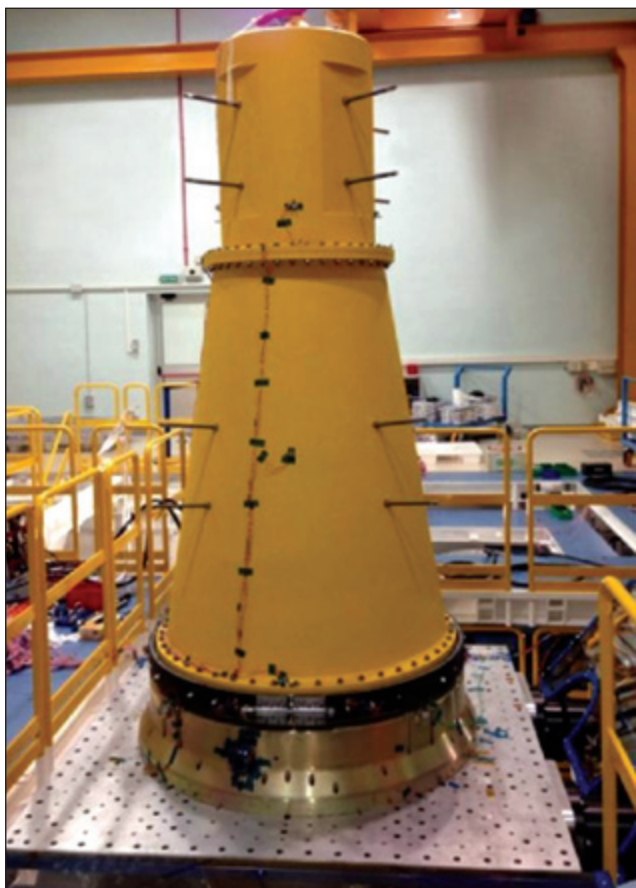
Figure 3. Typical four-ton dummy load used during system checkout.
